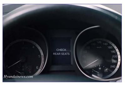
the system detects movement in the rear seats after the driver leaves the vehicle, the vehicle will honk its horn, flash lights, and send a message to the driver's phone. The alert system will be adopted in 2019 model year vehicles. More information on the system can be found at: <a href="https://www.hyundainews.com/en-us/releases/2383">https://www.hyundainews.com/en-us/releases/2383</a>
